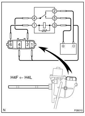
H4L (4WD and Center diff. lock "LOCK") → H4F (4WD (b) and Center diff. lock "FREE") shift:
