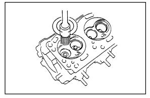
(b). Using a wire brush, remove all the carbon from the combustion chambers.
