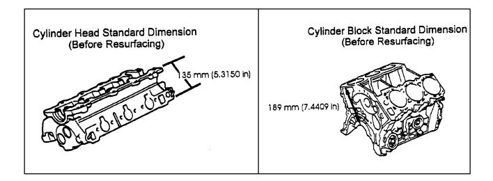
Always thoroughly clean a head or block that has been machined to ensure that all residue from the machining operation is completely removed.
