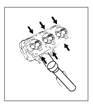
(b) Examine the intake and exhaust ports for signs of the solvent leaking past the valve seats, paying particular attention to cylinders number one and number six. If any solvent leakage is detected those valves must be removed for further inspection and repair as necessary.
